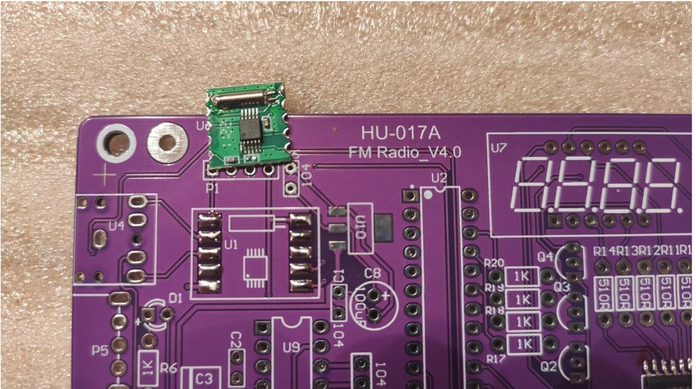
Solder this Radio module on the pcb.
