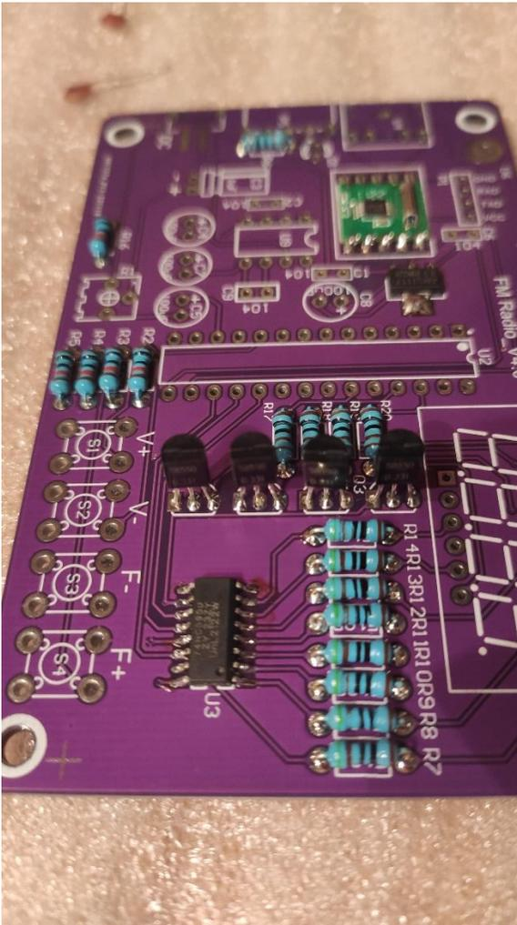
Be careful while soldering the transistors on the PCB, they need to be cooled a bit during the soldering process!
