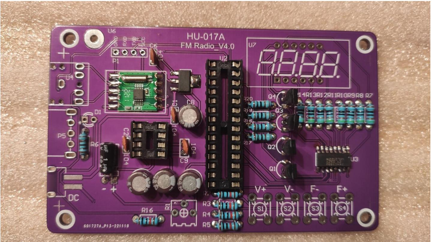
After the ELco's Solder also the IC base sockets for item U2 and U9.
