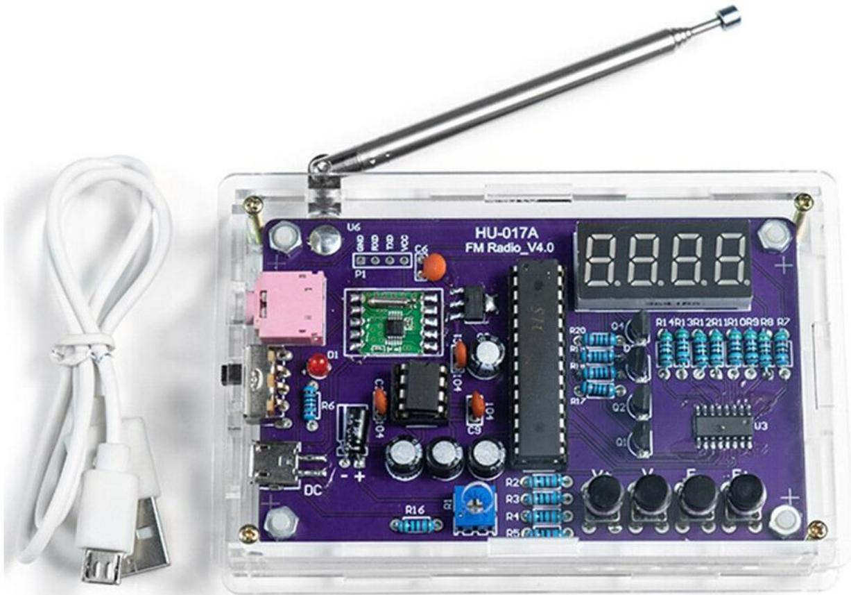
With this FM Radio, when it is finished, you can listen to several radio stations transmitted by air in the frequency range of 87-108MHz. So all your favorite stations on this small device!
