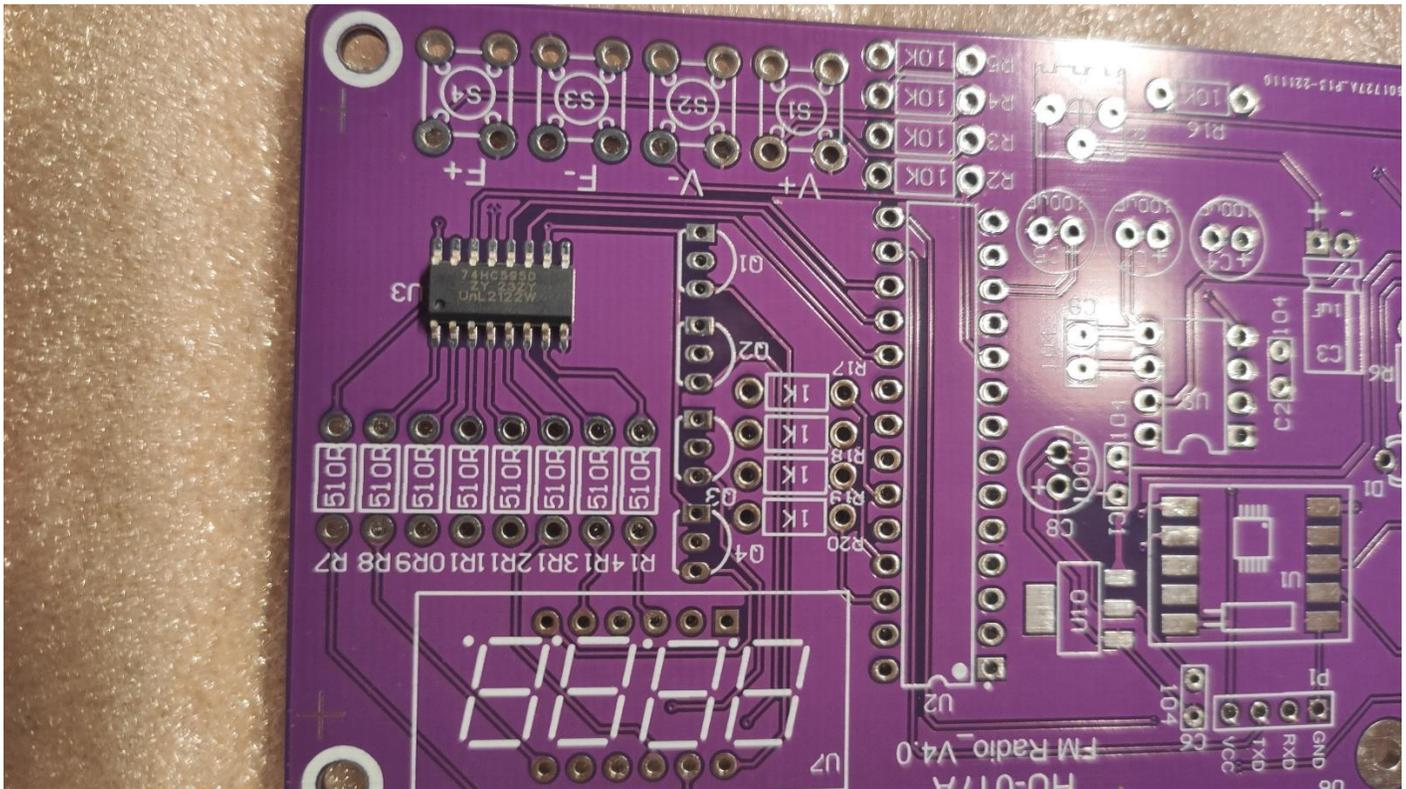
Be sure that the IC 74HC595D is positioned like the picture. Once you have soldered this one wrong it is a disaster to remove and resolder!!
